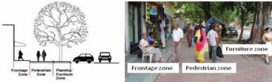
Figure 40 - Picture showing the division of Footpath/ Sidewalk into 3 zones
