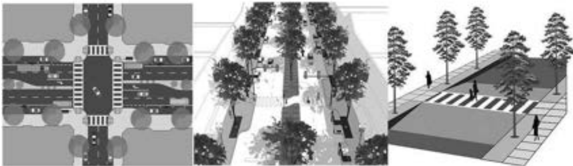
Figure 37 - Example for typical intersection crossing, midblock crosswalks to cross the streets with long distances between intersection crossings, raised cross walk
